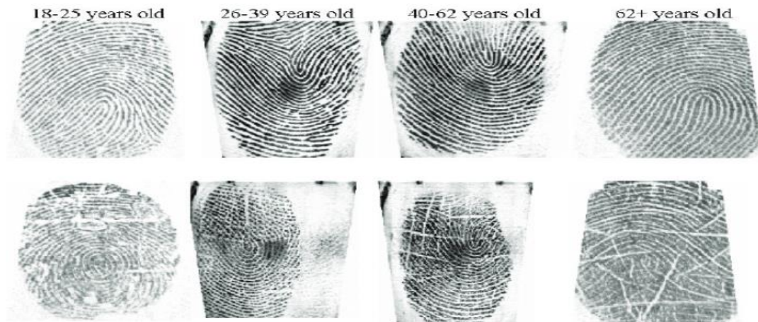
Figura 1: Samples of high quality fingerprints (top row) and low quality fingerprint (bottom row) with different age ranges.
